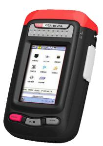
performance test and PPPoE function, FTP download and WEB browsing. At the same time, it provides a large amount of Ethernet diagnosis tools (PING, traceroute, port positioning tool, loop back tool etc.) , which satisfies the needs of Ethernet wiring test, bandwidth verification etc. in most cases.
